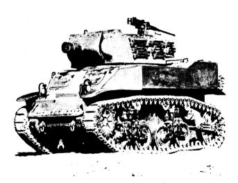
Figure 2. Carriage, motor, 75-mm howitzer.
